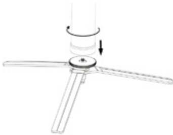
Foldable floorstand with 1/4"-20 thread
